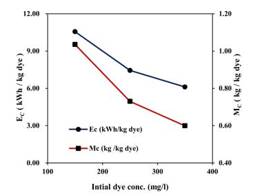
Fig. 8. Effect of initial dye concentration on energy and electrode consumption: volume of solution = 1 liter, NaCl Concentration = 1 g / l, applied voltage = 10 V, initial pH =  $7 \pm 0.5$
