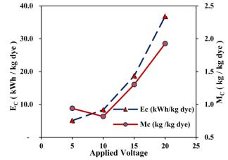
Fig. 4. Effect of applied voltage on energy and electrode consumptions: initial dye concentration = 250 mg/l, volume of solution = 1 liter, NaCl Concentration = 1 gm / l, initial PH = $7 \pm 0.5$
