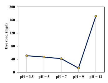
Fig. 6. Effect of initial pH on the final dye concentration: initial dye concentration= 250 mg/l, volume of solution = 1 liter, NaCl Concentration = 1 gm. / l, applied voltage = 10 V, EC treatment time = 15 min.
